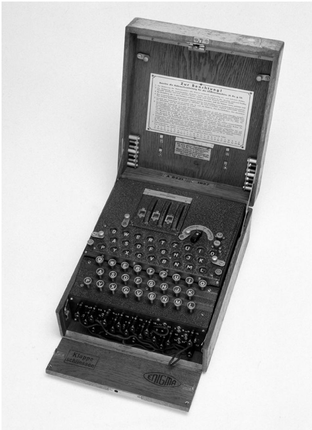
Figure 2. A three-wheel Enigma with the plug-board (at the front of the machine) exposed. The lampboard is behind the keyboard. The three wheel-slots are visible behind the lampboard. Beside each wheel-slot is a window through which letters marked on the wheels are visible to the operator.
